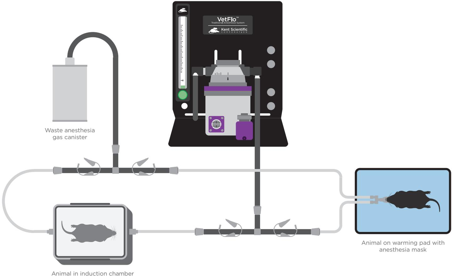
Perfect for laboratory and veterinary anesthesia delivery, the VetFlo vaporizer is completely self contained and portable. The multi-channel base is designed for multiple stations that are individually controlled. You can work with up to six stations, operating off of one vaporizer. With an easy-to-follow chart, each station can deliver a different flow rate of anesthesia.
