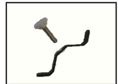
**For mid-size syringes** – Use the straight clamp. Secure the clamp with the central screw.
